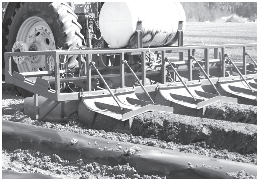
Fig. 2.6. Mulch laying after plowing to improve drainage.
